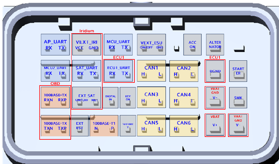
Fig. 3.7 Main Connector PINMAP1
