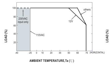
$\bigcirc$  If ELG-200 operates in Constant Current mode with the rated current, the maximum workable Ta is 50  $^{\circ}\mathrm{C}$  for 12V-model whereas 60  $^{\circ}\mathrm{C}$  for other models.
