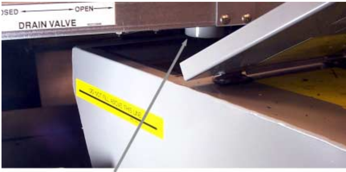
SDU properly positioned under fryer drain
