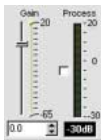
Figure 3.58. Process gain adjust and meter
