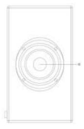
6. Passive Radiators: Two 5.25" passive radiators (one on each side).
