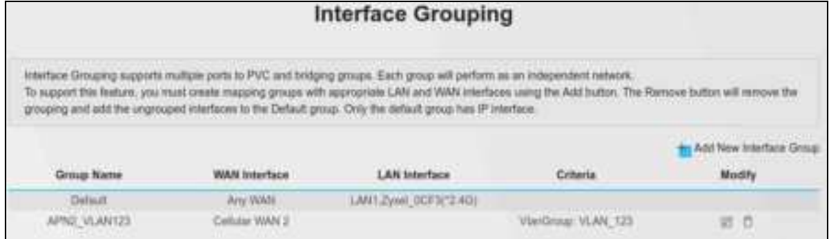
Figure 145 Network Setting > Interface Grouping
