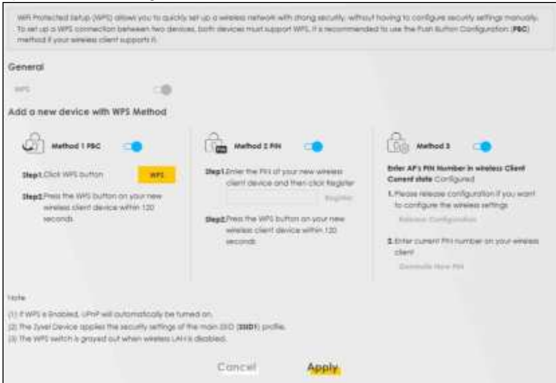
Figure 89 Network Setting > Wireless > WPS
