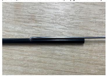
E. Slide the heat-shrink tubing over the piano wire and pushrod tube and heat to shrink and secure. Repeat the process on the other end and secure the 2mm nuts and clevis on the thread. Complete the final assembly of pushrod by adjusting to the required length of 470mm.
