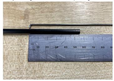
D. Insert the hook of the piano wire into the pushrod tube (as here), and secure on a skim of epoxy glue. Allow to dry.
