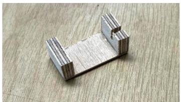
27. Fit your servo as below ensuring the servo horn is centred. Make sure you drill a pilot hole for the screws or you risk splitting the wood.
