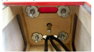
□ 30. Use masking tape to cover the motor and, using a dremel cutting disk, cut the rear of the shaft as below. This also needs to be done with the bolts that secure the motor.
