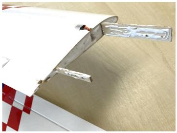
16. Glue the wing locating dowel into the belly pan and remove the film to reveal the wing bolt position.
