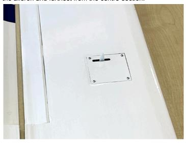
13. Using two of the four M2 piano wire pieces, introduce a Z-bend to the non-threaded end then add a clevis, nut and keeper to the other. The pushrods need to be approx.
