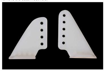
$^{\rm o}$  25. Using the pushrod to align the control horn on the elevator, mark the positions of the fixing holes whilst making sure that the pushrod is centralised down the fuselage. As before, make sure that the clevis attachment point is directly above the hinge line. When happy, secure the control horn using the 2mm bolts, backing plate and 2mm nuts. Cut off any excess thread that projects beyond the nuts and apply a small amount of glue to lock the nuts in position.
