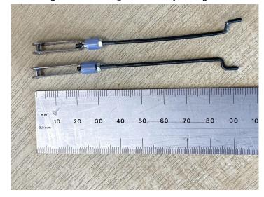
14. Ensuring your first servo and aileron are centred. Use the pushrod to position the aileron control horn so that the Z-bend is positioned over the aileron hinge point. Secure the control horn in place with the supplied screws. Repeat the process on the other wing.
