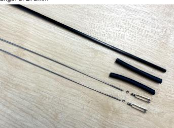
B. Measure 55mm from either end and drill a small hole through one face of the pushrod tube (not all the way through) to allow the 2mm piano wire pieces to hook into the tube.
