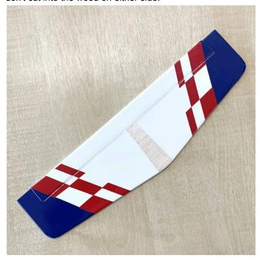
22. Slide the tailplane back into position and slot the fin in place. Mark the mating surfaces, as before, and remove the film where the fin will be glued to the fuselage. With the wing attached dry fit the tailplane and fin and look down the nose to ensure all is square. Adjust as necessary then glue the tailplane in position. Allow the glue to cure, fit the fin, check for alignment with a square, then glue in place.
