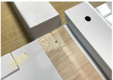
19. Put the wing and belly pan back on the fuselage and check to ensure that the wing bolt marries with the capture nut. When you're happy, remove the bolt and belly pan, apply glue to the contacting belly pan and wing surfaces, refit, secure with the wing bolt, and allow to dry.
