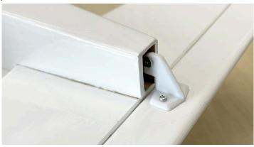
26. Using the two remaining and servo mounting blocks and base plate (elevator), glue together to make the elevator servo cradle.
