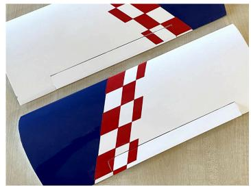
4. Hold the wing as shown and, using thin cyano, wick the glue into the hinge and balsa in exactly the same way as you did in Step 2.
