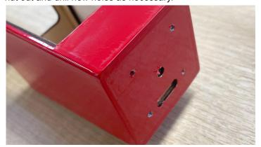
**Warning:** Before installing the motor of your choice we recommend you ensure nothing projects into the battery bay area. Bolts and motor shaft should be cut so as not to project into the battery area.
