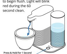
**6.** Once the flush is complete, light blinks blue for 5 seconds, then illuminates solid blue for 5 seconds.
