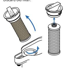
2. Remove plastic from new filter. Press new filter into filter chamber cap
