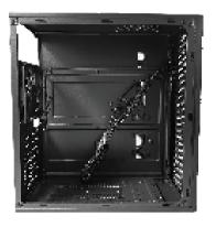
Place the HDD/SSD in the HDD/SDD slot provision and fix it with screws.
