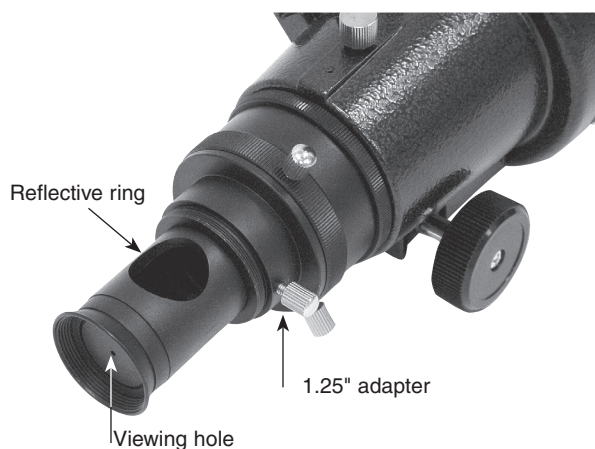
Figure 6-1. The collimating tool in the StarSeeker 100 focuser.
