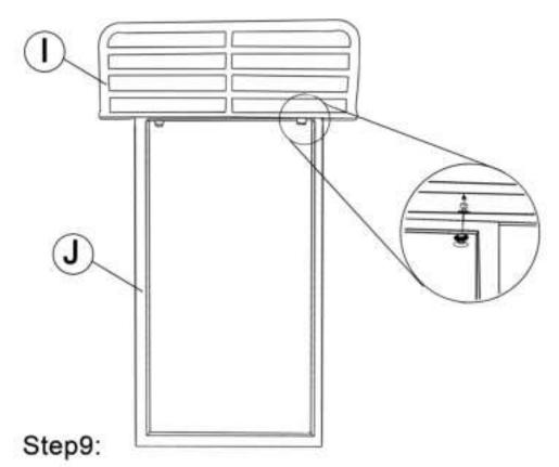
Installing the footrest by connecting part (I) and (J). Using 2 screws - M6,30mm
