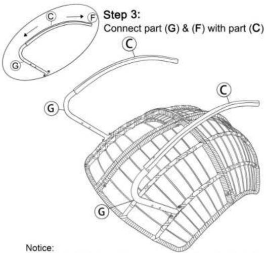
1-Please don't tighten all screws completely at beginning! 2-Fully tighten after completing the chair!
