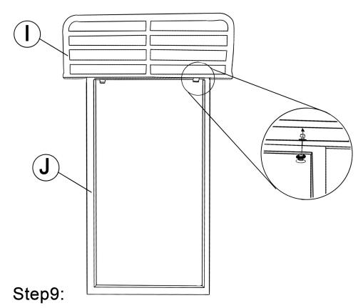
Installing the footrest by connecting part ( $\mathbf{I}$ ) and ( $\mathbf{J}$ ). Using 2 screws - M6,30mm
