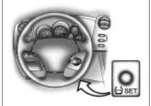
Press and hold the tire pressure warning reset switch until the tire pressure warning light flashes slowly on/off three times. Wait for a few minutes with the ignition in ON/RUN, and then turn the ignition to ACC/ACCESSORY or LOCK/OFF.
