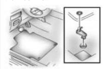
To remove the floor mat, pull up on the rear of the mat to disconnect it from the locator books.
