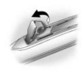
Push the release lever and slide the wiper assembly toward the driver side of the vehicle.
