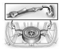
3. Use the tire tie-down straps located under the floor panel to secure the flat tire.
