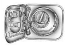
The tethered fuel cap is located behind a hinged fuel door on the driver side of the vehicle.
