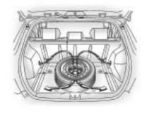
5. Pass the straps through the center hole of the wheel.
