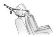
If the position you are using has an adjustable headrest or head restraint and you are using a dual tether, route the tether around the headrest or head restraint.
