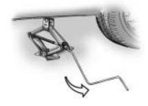
Turn the jack handle counterclockwise. Lower the jack completely.
