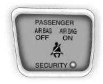
The words ON and OFF will be visible during the system check. When the system check is complete, either the word ON or the word OFF will be visible depending on
