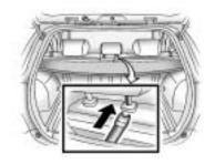
4. Attach the center hook to the center head restraint.
