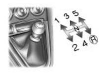
**1 (First):** Press the clutch pedal and shift into 1 (First). Then, slowly let up on the clutch pedal as you press the accelerator pedal.
