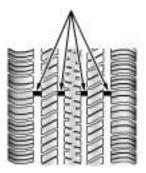
One way to tell when it is time for new tires is to check the treadwear indicators, which will appear when the tires have only 1/16 inch (1.6 mm) or less of tread remaining. You need new tires if any of the following statements are true:
