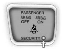
The security light, located on the center of the instrument panel, comes on if there is a problem with arming or disarming the theft-deterrent system.
