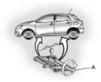
Position the jack and raise the jack lift head to fit over the car flange between the two notches.
