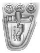
The shift lever is located on the console between the seats.
