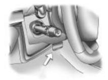
The adjustment lever is located on the left side of the steering column.
