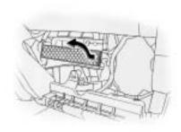
2. Push the side fastener to release and remove the filter cover.
