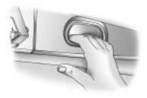
Close the liftgate by using the handle to pull it down.
