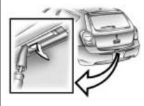
Press the tabs in to disengage them and remove the license plate lamp assembly.
