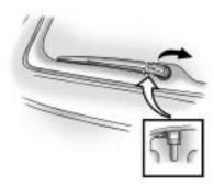
Disengage the two pins and disconnect the rear wiper arm by pulling them up.
