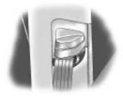
Push down on the release button and move the height adjuster to the desired position. The adjuster can be moved up by pushing on the front of the height adjuster. After the adjuster is set to the desired position, try to move it down without pushing the button to make sure it has locked into position.
