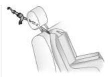
If the position you are using has an adjustable headrest or head restraint and you are using a single tether, raise the headrest or head restraint and route the tether under the headrest or head restraint and in between the headrest or head restraint posts.
