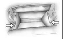
Open the glove box door. Push each side of the glovebox in and pull out to remove.
