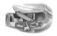
To release the parking brake, hold the brake pedal down. Pull the parking brake lever up until you can press the release button. Hold the release button in as you move the lever all the way down.
