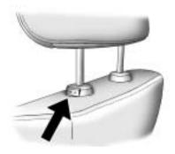
To lower the head restraint, press the button, located on the top of the seatback, and push the restraint down. Push down on the head restraint after the button is released to make sure that it is locked in place.
