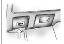
Pull the release handle, located below the instrument panel to the left of the steering wheel.
