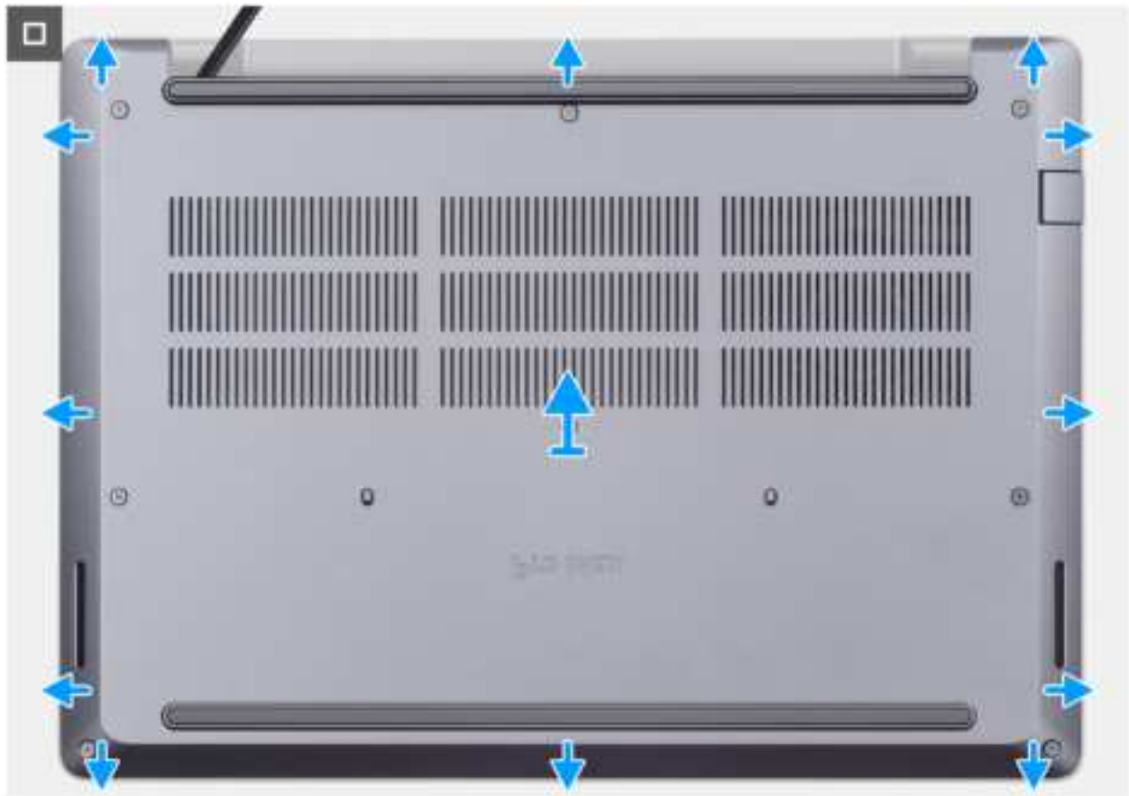
Figure 12. Removing the base cover
