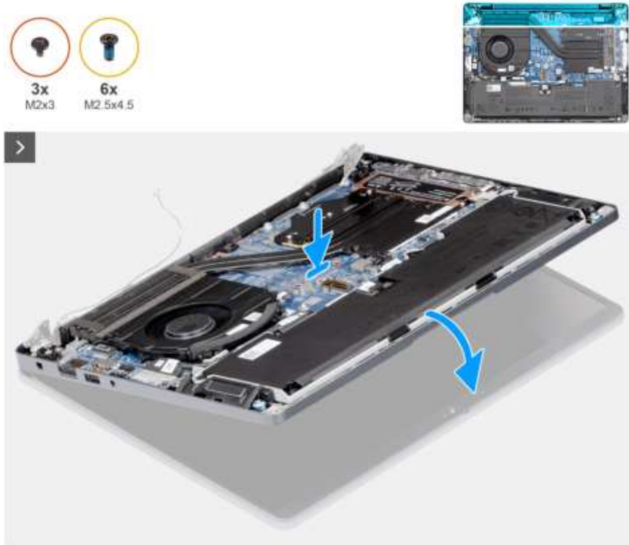
Figure 47. Installing the display assembly
