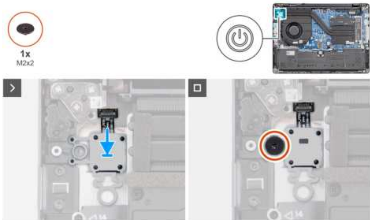
Figure 43. Installing the power button
