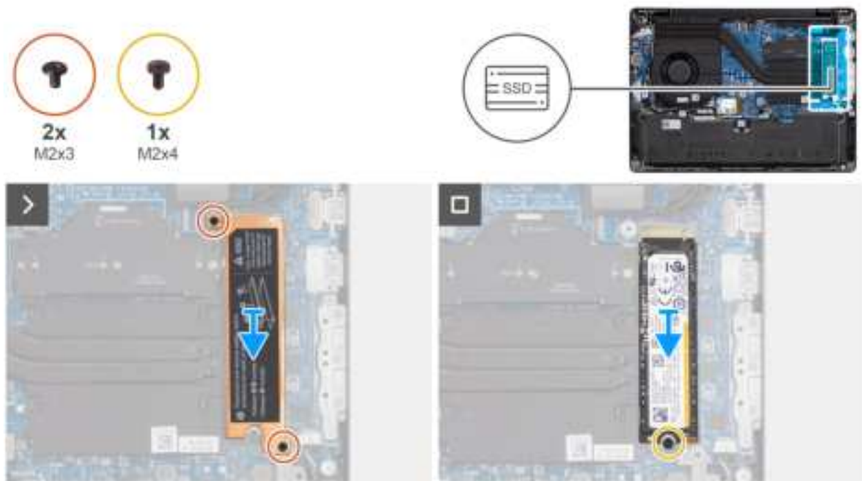
Figure 22. Removing the M.2 2280 solid state drive
