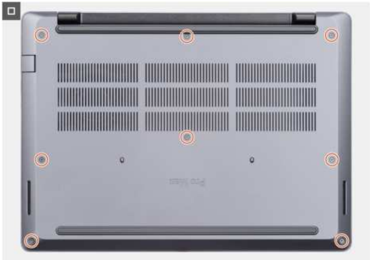
Figure 15. Installing the base cover
