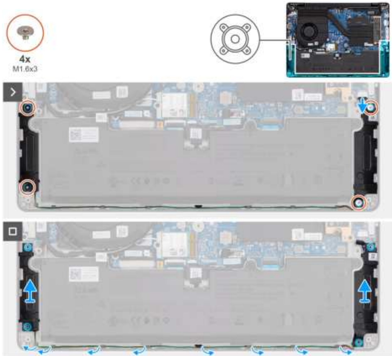
Figure 26. Removing the speakers
