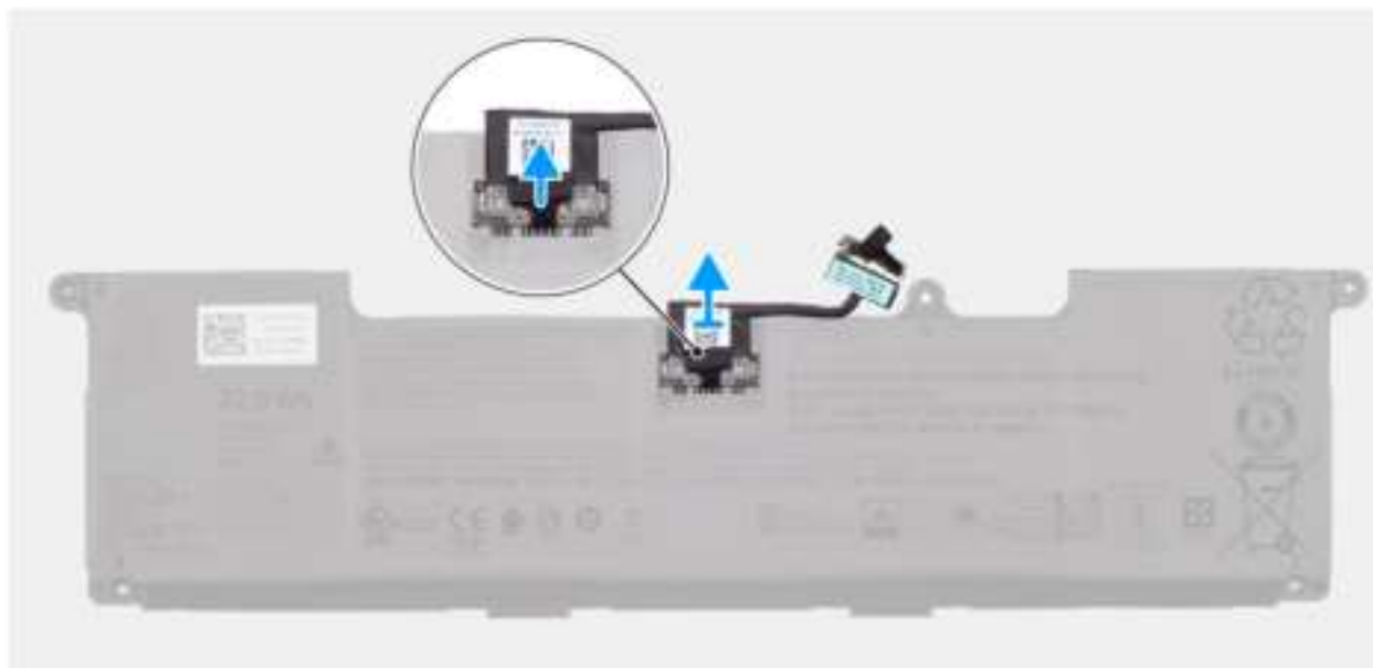
Figure 31. Disconnecting the battery cable
