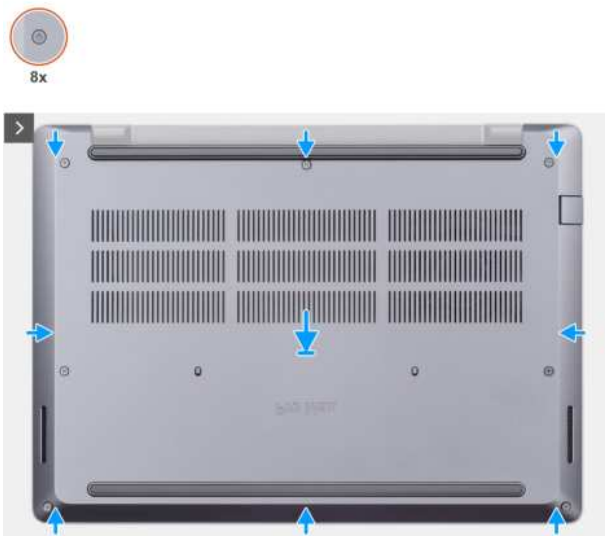
Figure 14. Installing the base cover
