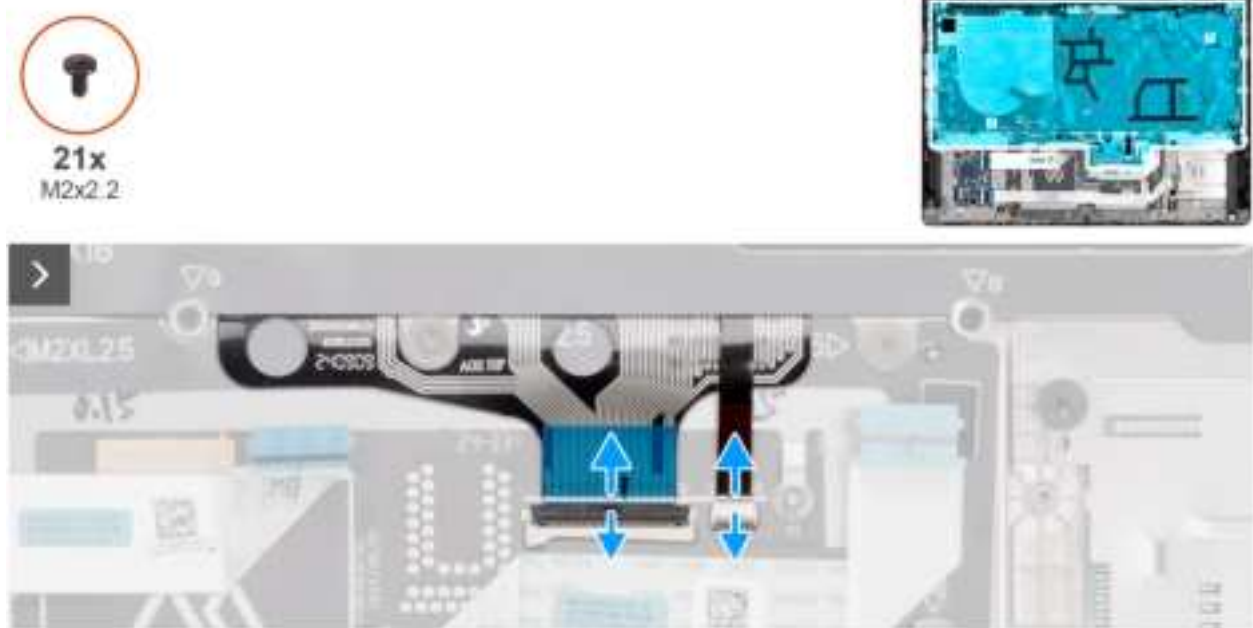
Figure 85. Removing the keyboard
