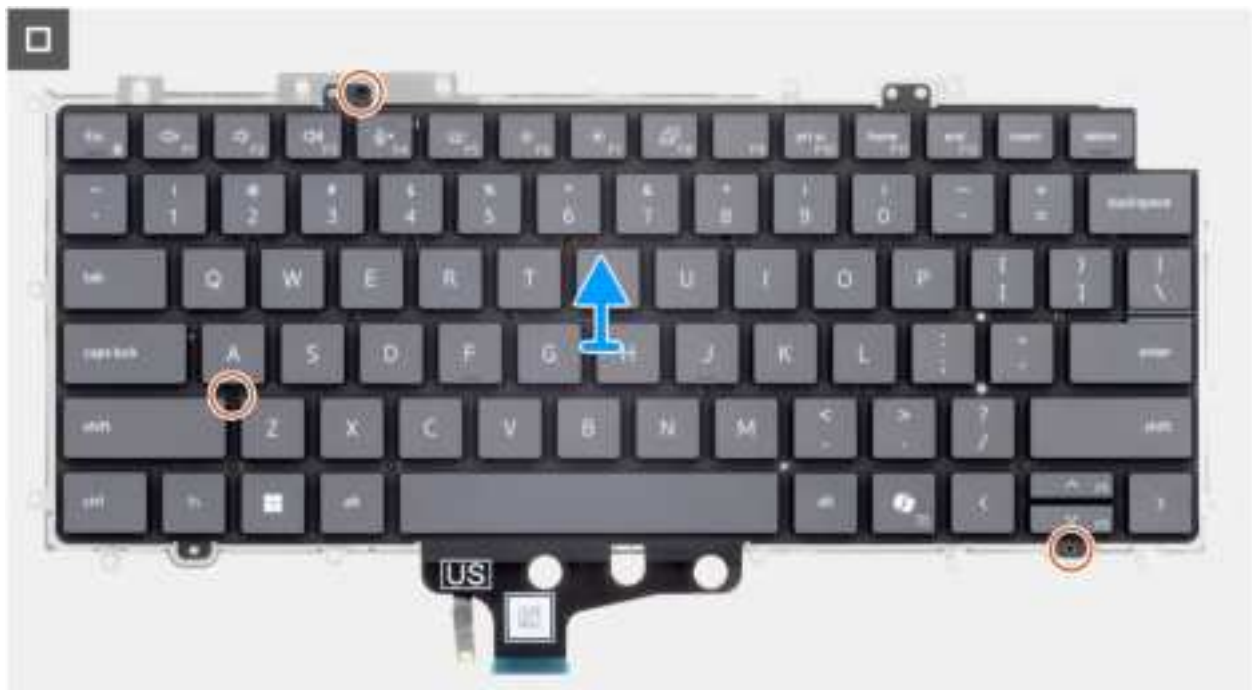
Figure 87. Removing the keyboard
