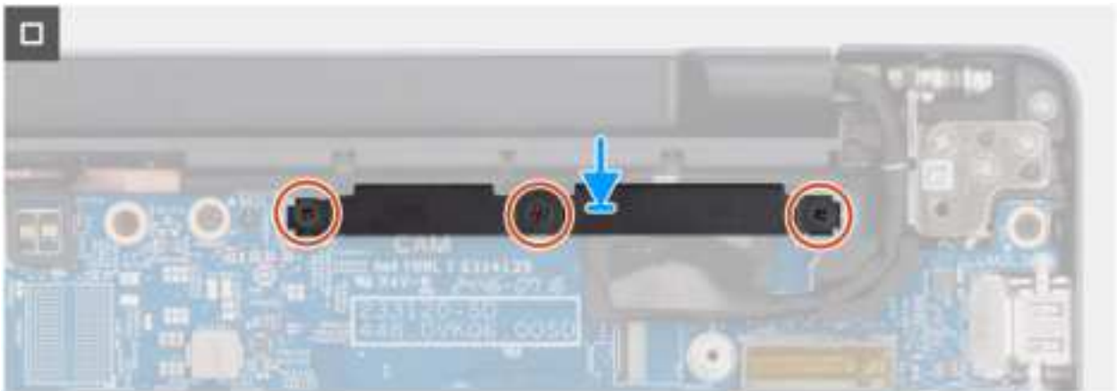
Figure 82. Installing the system board
