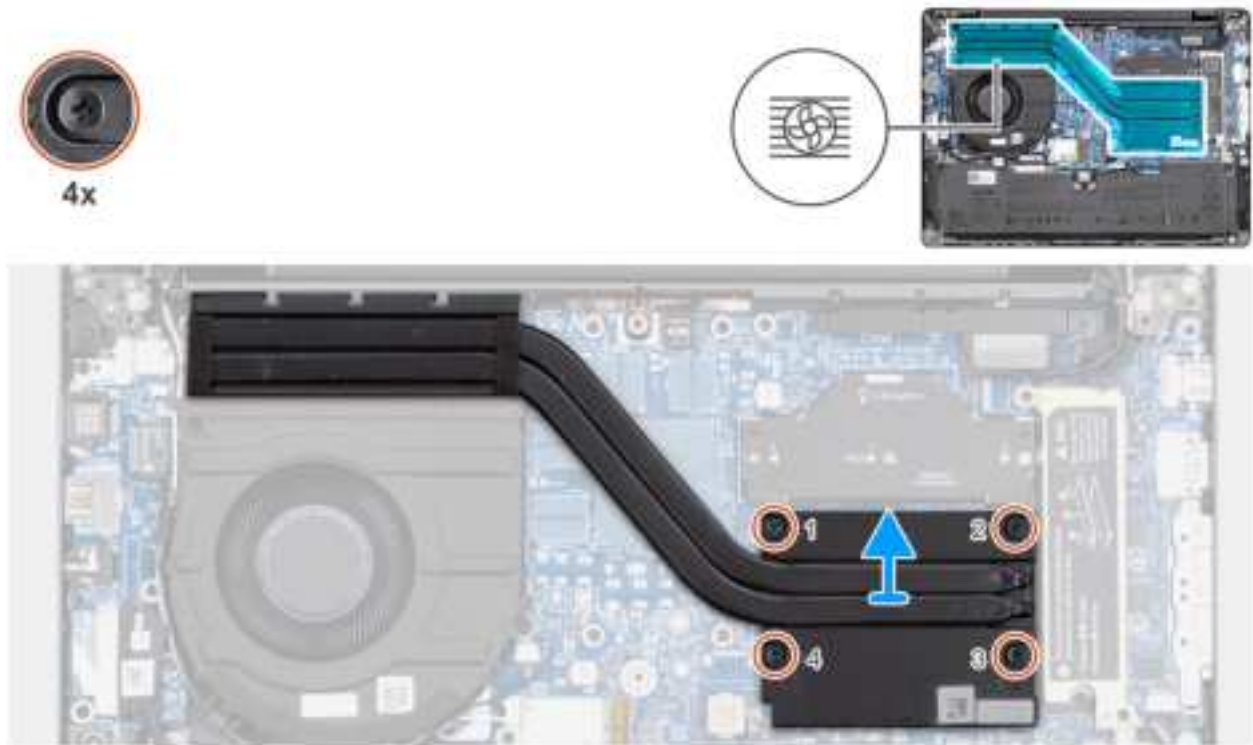
Figure 38. Removing the heat sink
