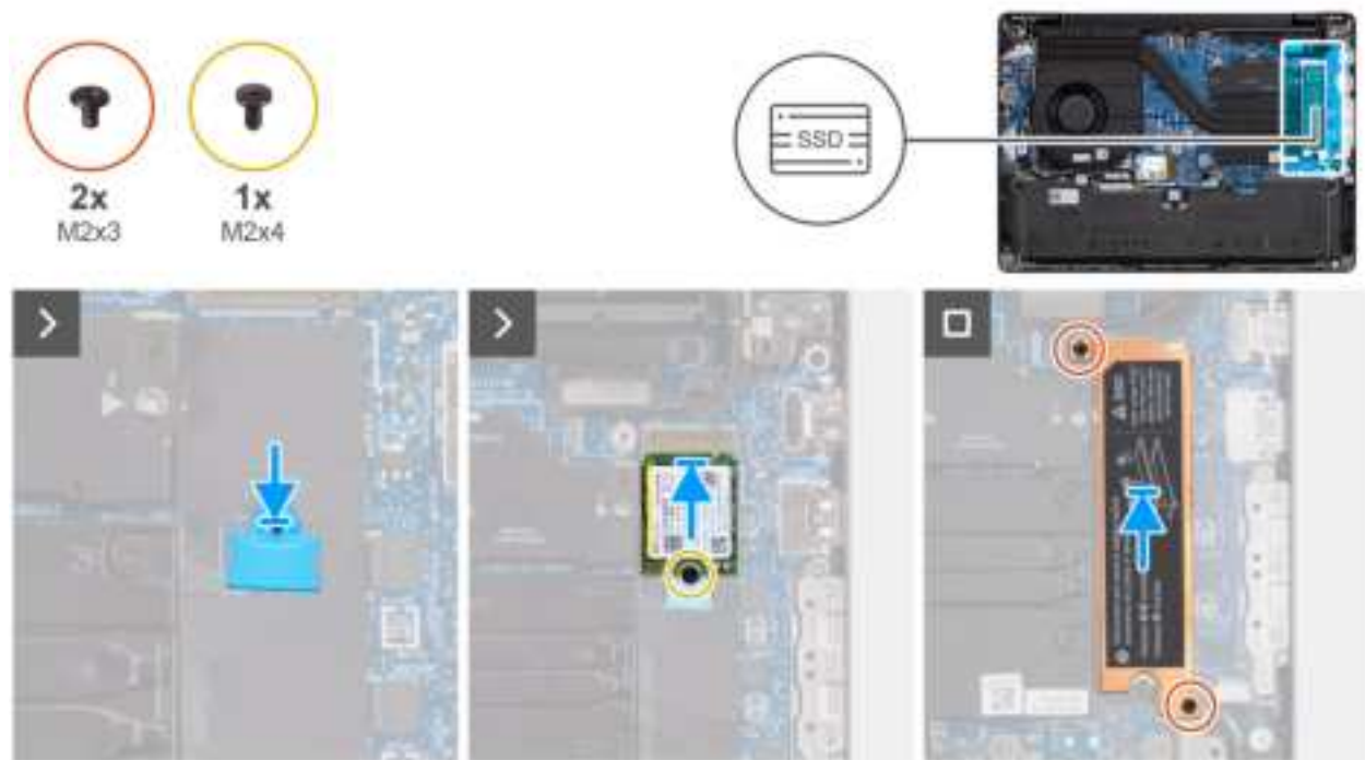
Figure 21. Installing the M.2 2230 solid state drive
