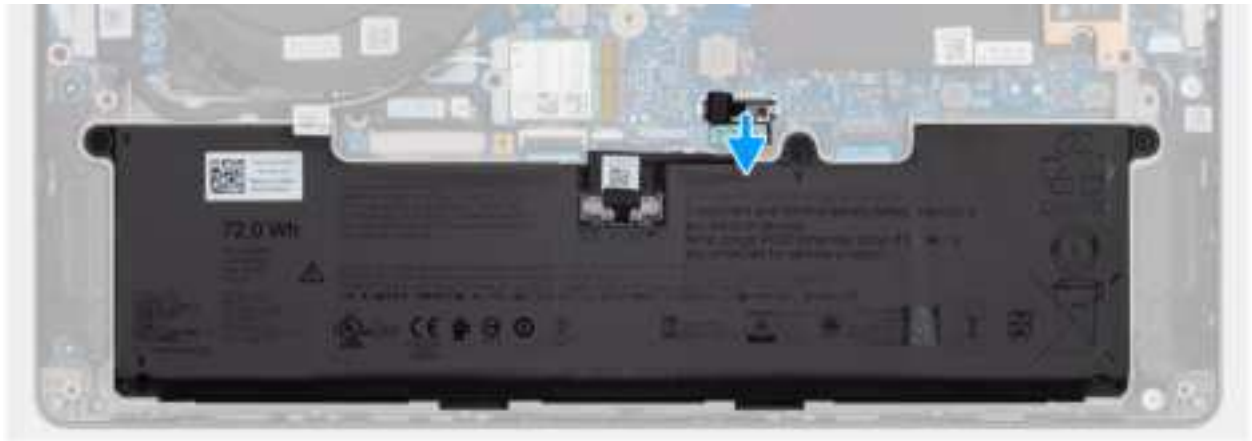
Figure 13. Removing the battery cable
