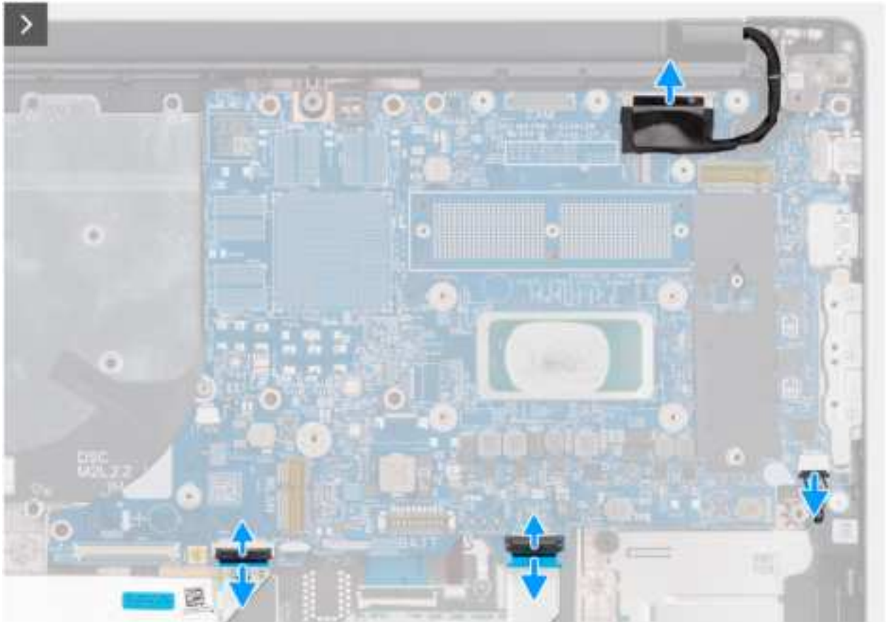
Figure 75. Removing the system board
