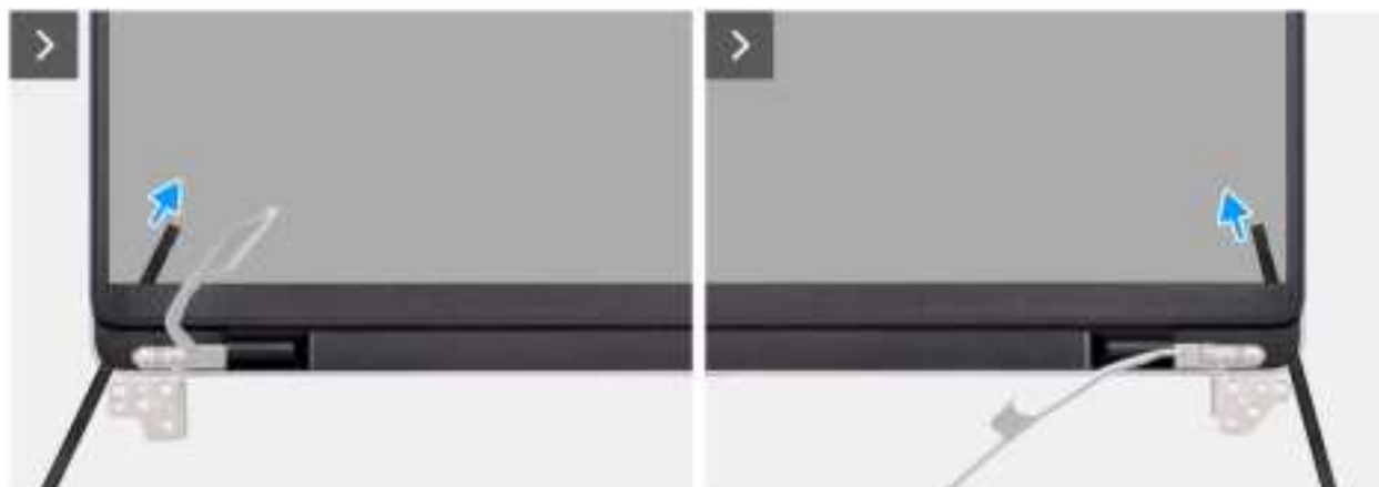
Figure 50. Removing the display bezel
