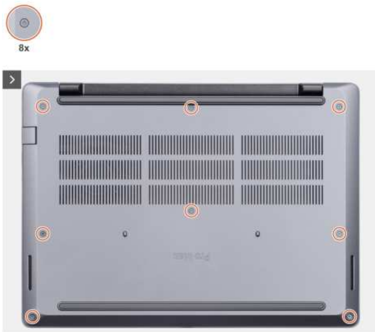
Figure 11. Removing the base cover
