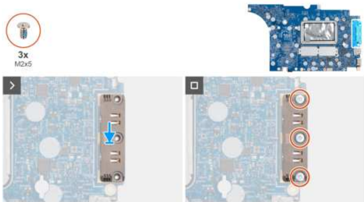
Figure 84. Installing the USB Type-C module
