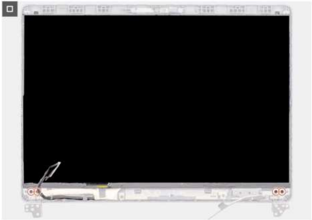
Figure 62. Installing the display panel
