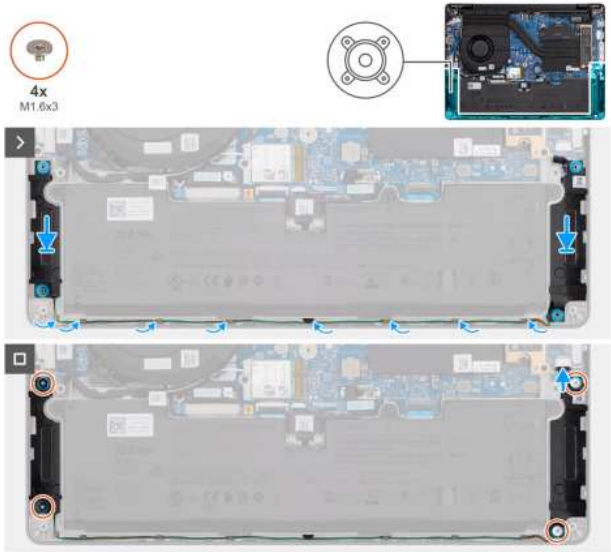
Figure 27. Installing the speakers
