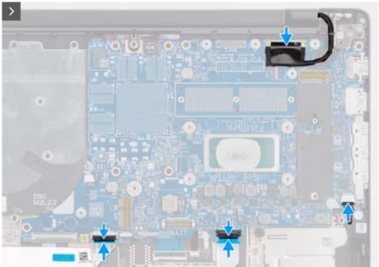
Figure 79. Installing the system board
