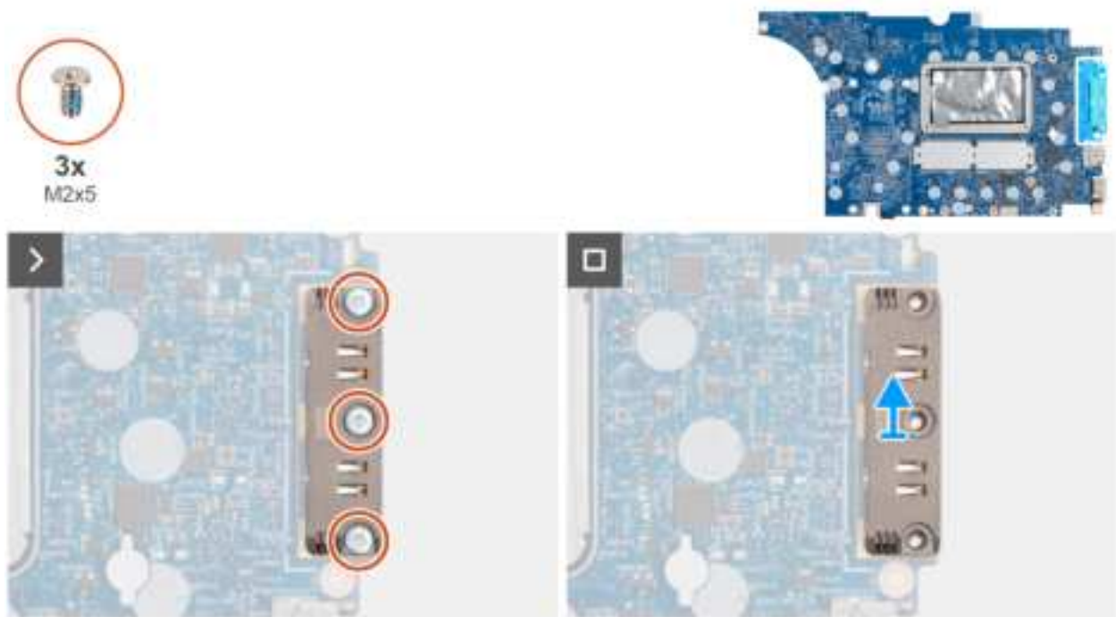
Figure 83. Removing the USB Type-C module
