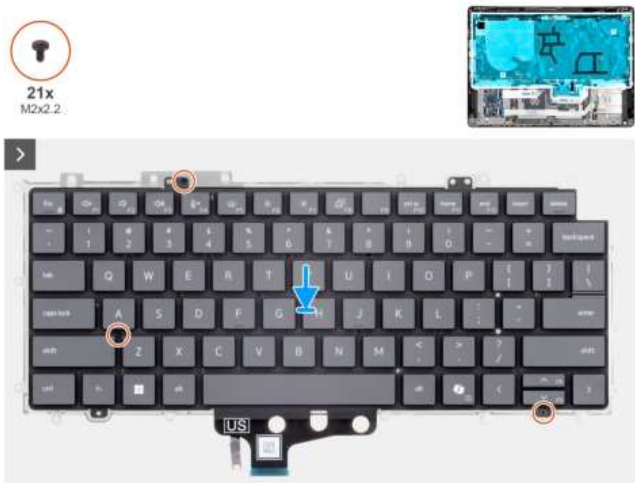
Figure 88. Installing the keyboard
