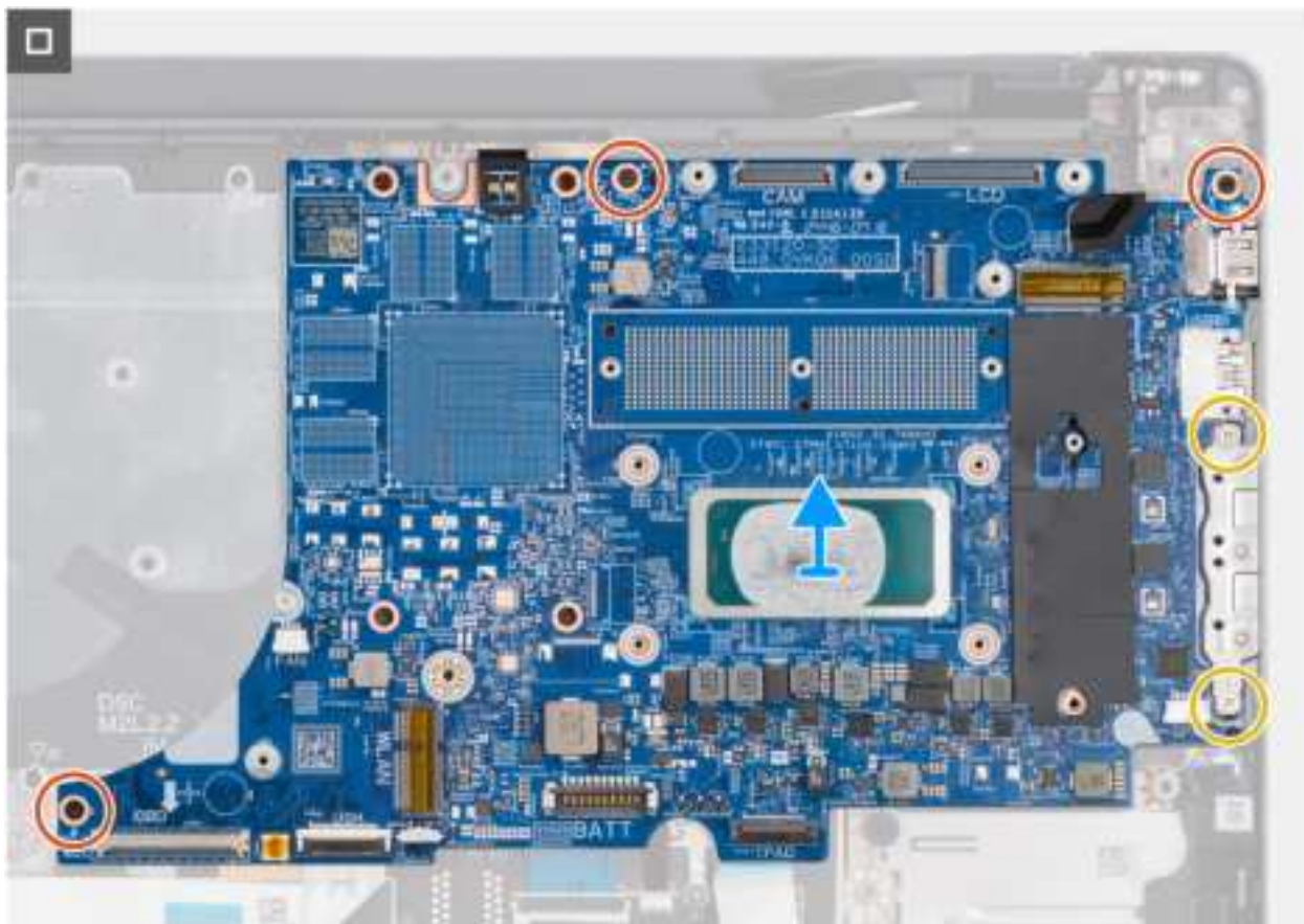
Figure 76. Removing the system board
