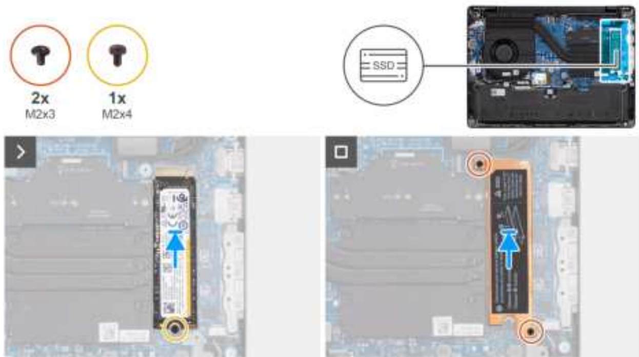
Figure 23. Installing the M.2 2280 solid state drive
