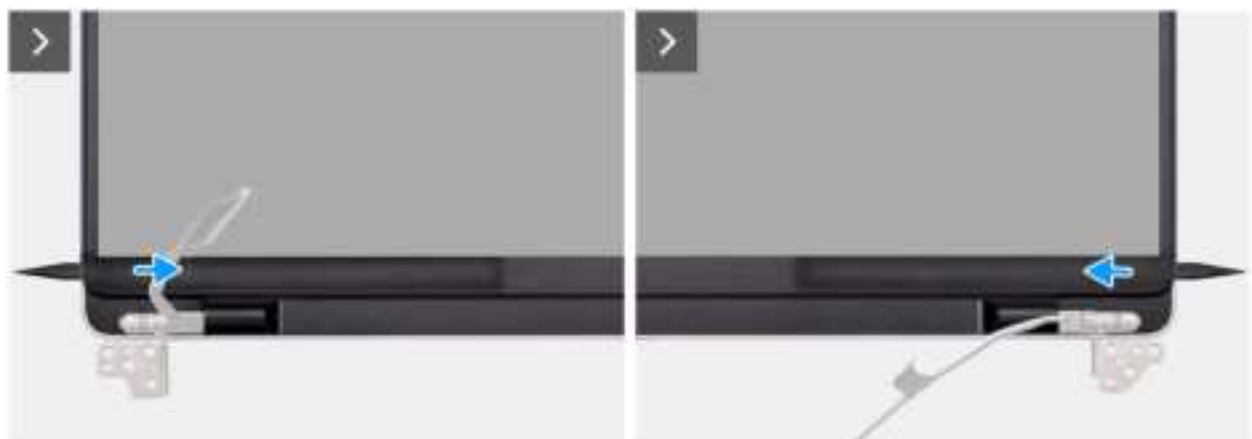
Figure 53. Removing the display bezel
