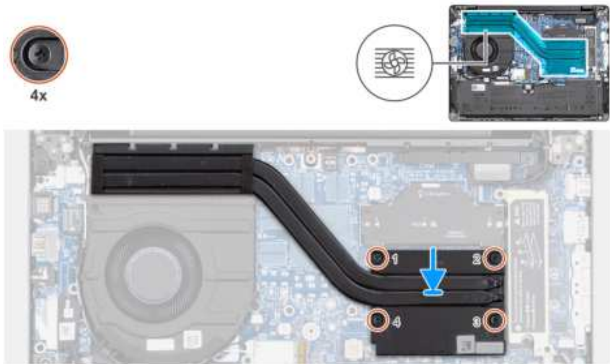
Figure 39. Installing the heat sink
