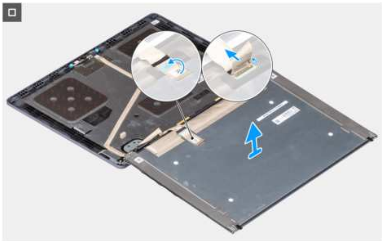
Figure 59. Removing the display panel
