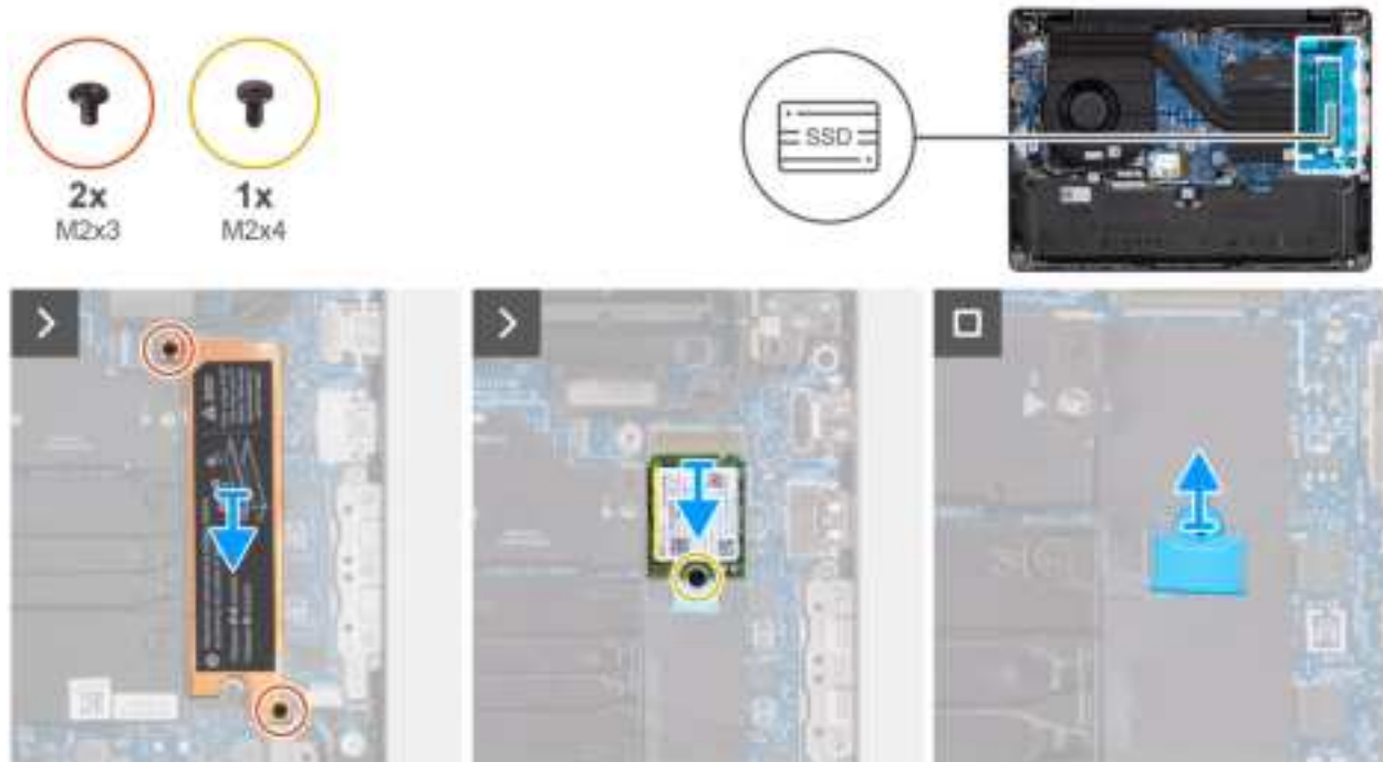
Figure 20. Removing the M.2 2230 solid state drive
