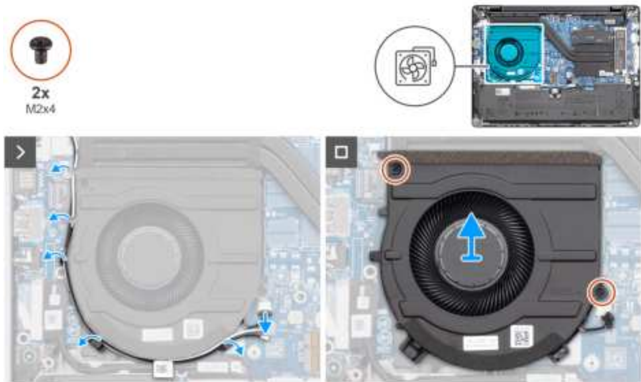
Figure 29. Removing the fan
