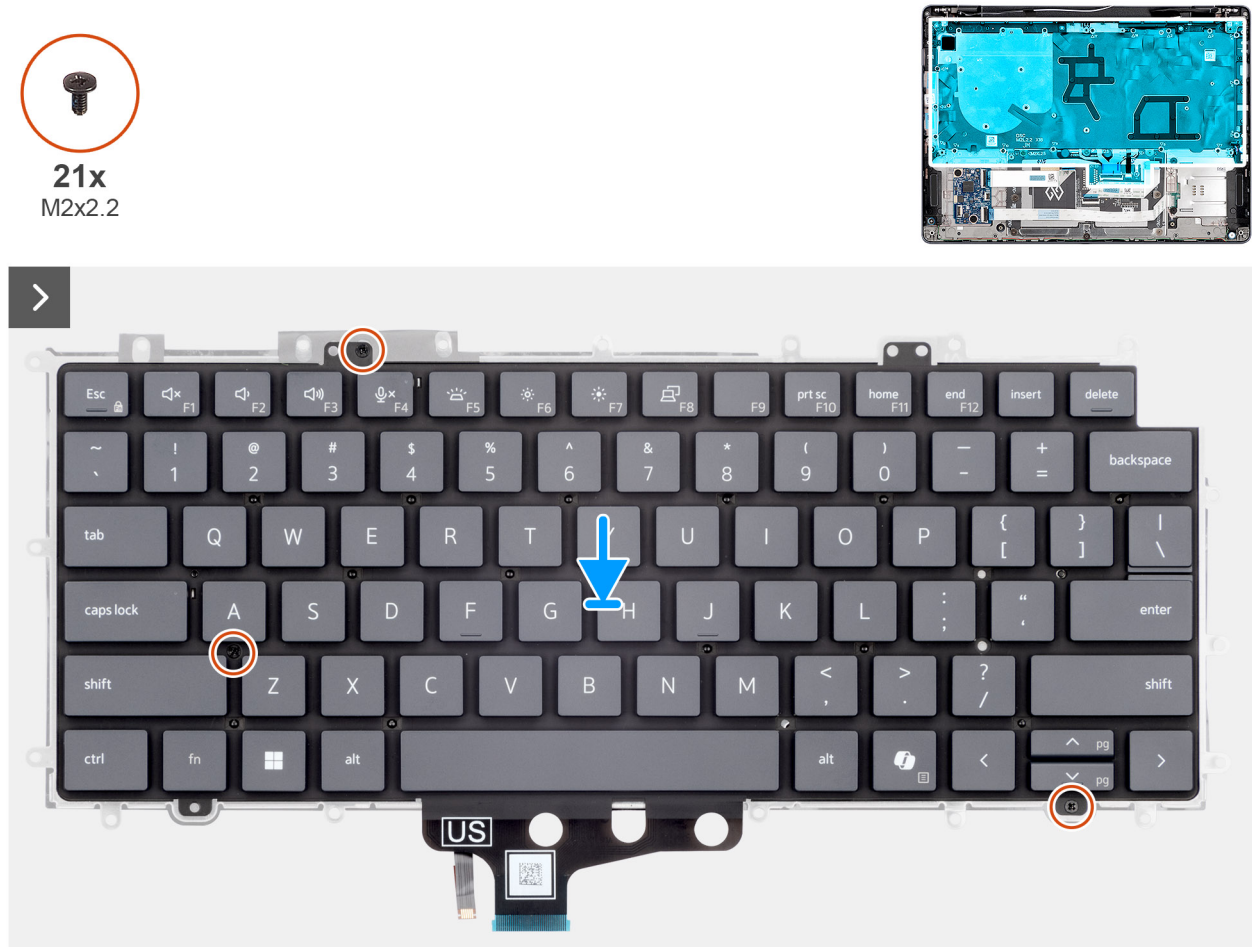
Figure 88. Installing the keyboard
