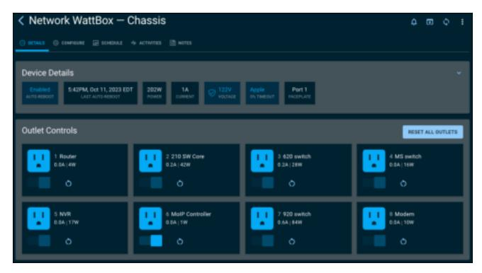
Note: If an outlet is set to **Disabled** you cannot control it. If an outlet is set to **Reset**Only it can only be reset.
