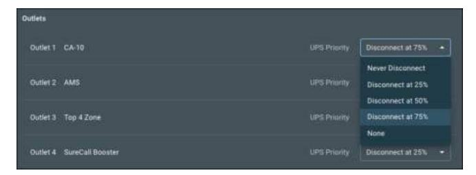
**Note:** Load shedding does not work for outlets configured to **Reset Only**.
