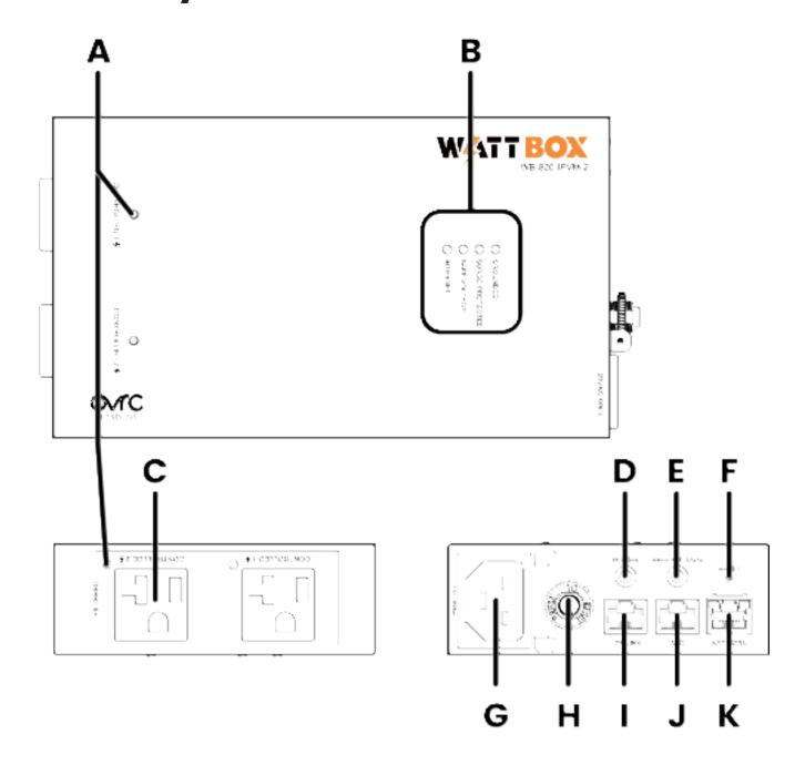
A. **Power indicators for outlets 1-2** —Illuminates when power is on (\*2 – 1 for each outlet).
