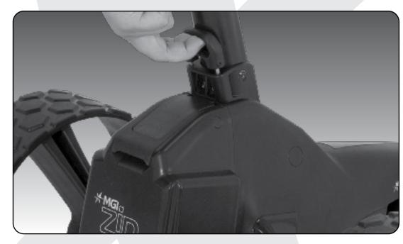
**Step 3:** Pull the latch up at the bottom of the handle.
