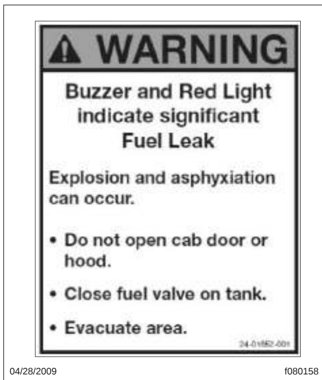
Fig. 19.5, Exterior Warning Sticker
