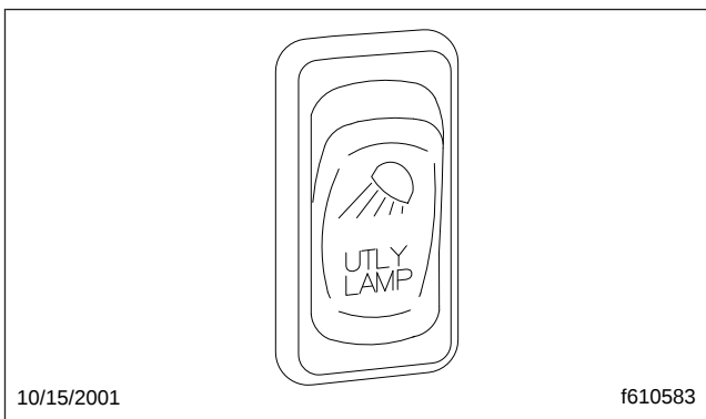
Fig. 5.10, Utility Light Switch
