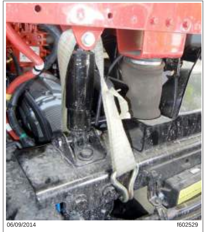
Fig. 24.7, Tension Strap Installed to Hold Down the Cab
