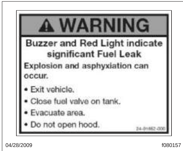
Fig. 19.4, Interior Warning Sticker
