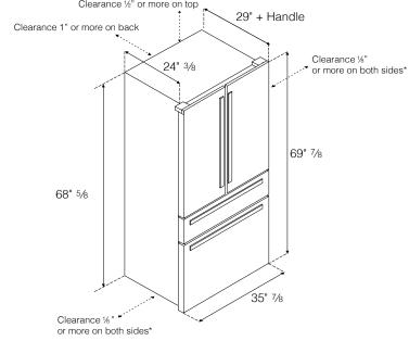
\* Added clearance for door opening swing might be needed based on adjacent cabinetry or wall structure.
