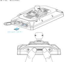
\*After installing the microSD card, firmly press the waterproof plug until it is flush with the body. Failure to do so may compromise waterproofing. \*安装 microSD 卡后,请将防水塞用力按压至机身平齐,否则可能影响防水效果。
