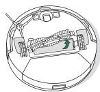
**3** Remove any hair or debris from the Multi-Surface Brush using the cleaning brush
