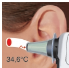
An obstructed view of the eardrum causes incorrect readings
