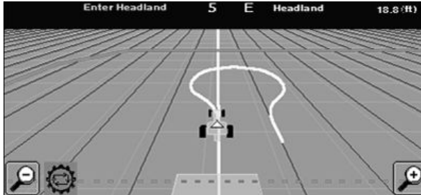
Symmetrical Light Bulb Turn (Control Point at 0 m (0 ft.) or Using 3-Point Hitch) (Turn Radius is Greater Than half of Track Spacing)
