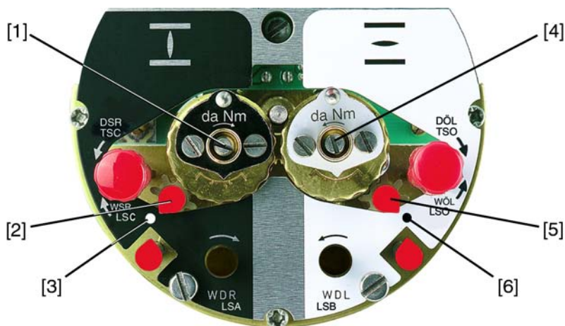
Figure 38: Setting elements for limit switching
