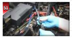
Plug the (B-H3741) Y-splitter, 2-Pin 14-AWG harness into the amplifier's subwoofer output plug. Route to both sides of the center console for the (250-MAVR-RUS10U) rear-seat subwoofer
