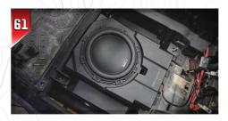
Using a **T35 Torx bit** and the provided screws from (B-HPM612HHW14-4) M6x12 Hex Head screws hardware pack, secure the enclosure to the seat's mounting brackets. Repeat for both subwoofers.
