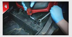
Slide the front drivers side seat back to expose the seat's front mounting bolts. Using a **13mm socket** and **wrench**, remove the nut and bolt from both sides of the seat.
