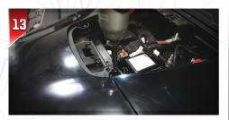
Remove the **Two (2) 10mm trim panel bolts** located beneath the dash panel you just removed.
