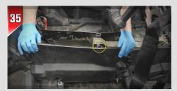
Remove the remaining console panels. Pull away from the center console to release the speed clips.
