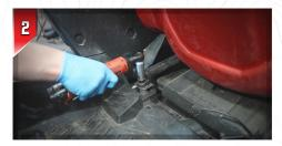
Using an **18mm Socket,** remove the bolts.
