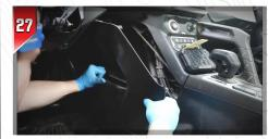
Remove the front drive side center console kick panel. Release the speed-clips by pulling the panel directly away from the center console.
