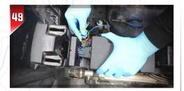
Route your amplifier's harnesses through the opening on the amp plate. Using the provided (B-S1157) M4 x 8 Phillips Pan-Head Screw, mount the amp onto the (2) mounting plates.
