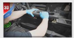
Remove the top cup holder panel by prying straight up. This will release the speed clips.
