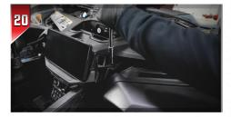
Remove the **eight (8) 10mm screws** securing the top panel in the dash.
