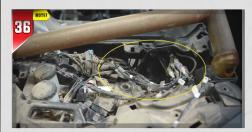
Locate the existing SSV Works amplifier assembly. Unplug the existing **SSV Works B-H3517 input to RCA harness** for the subwoofer amp (a small white MavR Audio plug).
