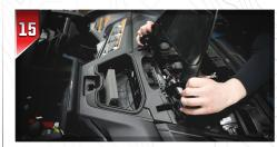
Open the upper storage compartment door and remove it by lifting straight up, this will release it from the hinges.
