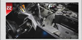
Remove the **three (3) 10mm screws** securing this panel.
