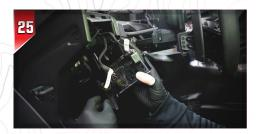
Pull the rocker switch cluster from the dash and remove the plugs from behind it.
