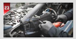
Remove the **Three (3) T30 Torx screws** on the side of the vehicle, just under the A-pillar. These are holding in the top dash panel.
