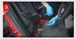
Using a **5/8 socket,** remove the bolts to the seat belt harness that attach the harness to the sides of the seat.
