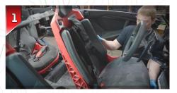
Slide the drivers side front seat all the way forward to expose the rear mounting bolts.
