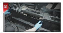
Remove the side plastic panels by releasing the speed clips puling away from the center console.
