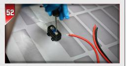
Using a Philips screwdriver, assemble the provided fuse and **8-AWG power wire** onto the fuse holder.
