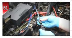
Plug the (B-H3741) Y-splitter, 2-Pin
