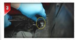
Unplug the driver's seat wiring harness, then pull the plug and its speed clip straight up to remove it from the center console.
