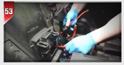
Route the power and ground cables from the amp to the battery through the opening in the center console. Leave the two terminals at the battery but not hooked up.
