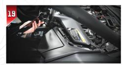
Then Remove the gloss black plastic trim panels around the dash. They are held in by speed clips you can pull toward the rear of the vehicle to remove them.
