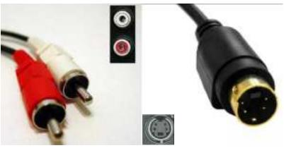
S-Video cables can transmit a higher quality video signal than regular RCA (Composite) cables, but they do not carry an audio signal. RCA (Composite) audio cables are still required when you are making an S-Video connection.
