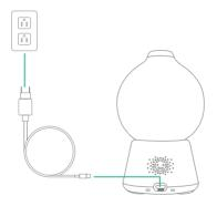
Slow flash of the red LED indicator suggests that the product has been powered on and that Wi-Fi configuration can be done.
