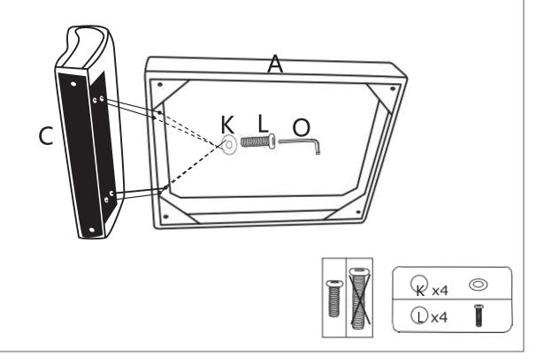
STEP 3 :Assemble the Right armrest (D) to the Seat frame (A) with the Washers (K) and the Bolts (L).
