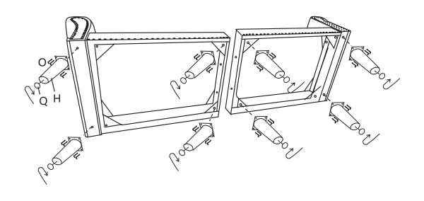
STEP 5 :Assemble the Seat frame (A) to the Seat frame (A) with the Butterfly nuts (N)  $\setminus$  Washers (K) and the Bolts (M).
