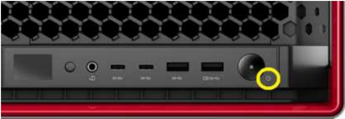
Figure 2 – Location of storage drive activity light
