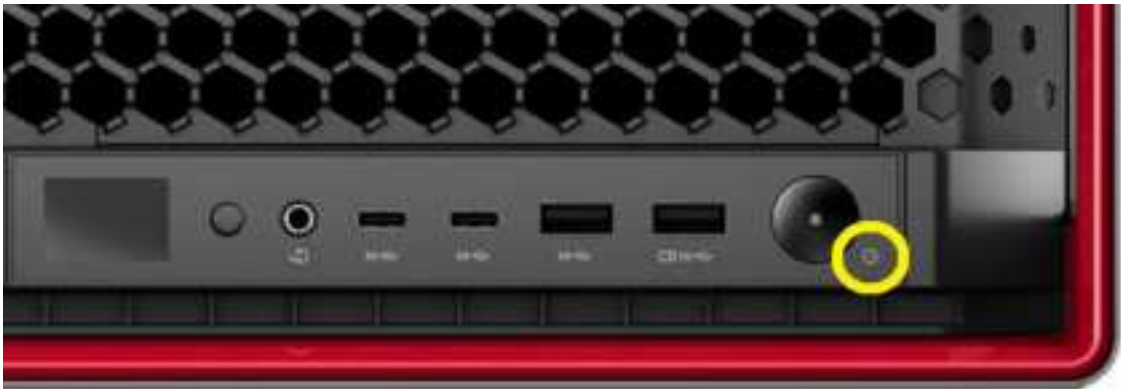
Figure 3 - Location of storage drive activity light
