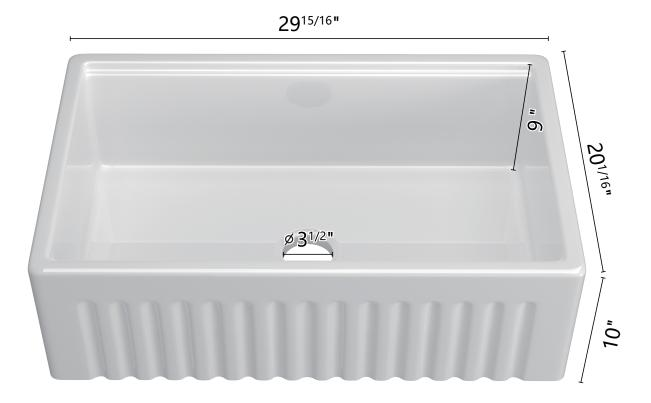
**KINDLY ATTENTION:** To present a perfect installation, please measure the actual sink size for the cutout and trace for the countertop. Do not cut the countertop until you receive the sink. Because this fireclay sink size may vary in size by up to 1/4 inch during the high-temperature firing production.
