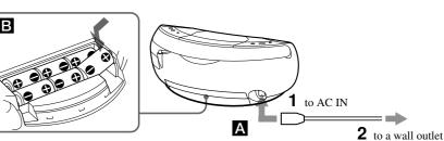
Connect the AC power cord A or insert six size D (R20) batteries (not supplied) into the battery compartment B.
