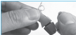
Figure 6. Insertion de la pile.
