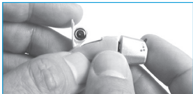
Figure 4. Open the battery compartment.
