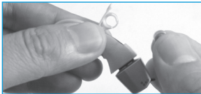
Figure 6. Insert the battery.
