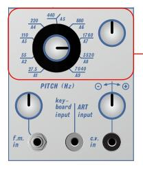
The **Principal oscillator's frequency knob** adjusts **octaves**, while the smaller knob handles fine up-tuning. To play the note center pitch, set only the fine-tune knob to the minimum.
