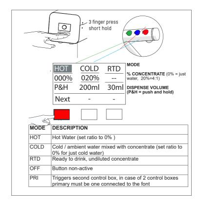
Volumes must be calibrated and machine must be notified of Chillers presence, refer to Control Box manual for futher instructions
