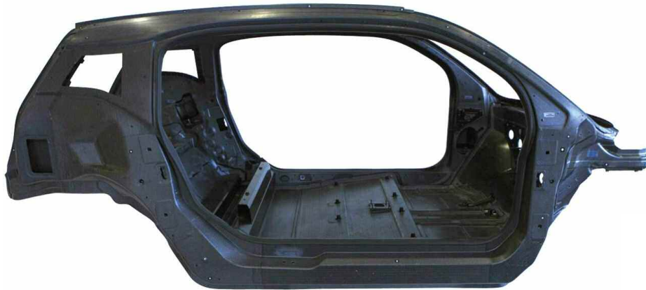
BMW i3 carbon fiber reinforced plastic (CFRP) life module
