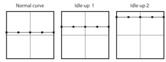
In governor mode, set the throttle curve to a horizontal straight line. Set the value according to the rotor speed.
