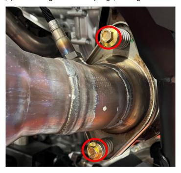
**Step 6:** Mark the lower exhaust mounting bolts for correct alignment when installing the new muffler. Remove (2) 13mm bolts once done.
