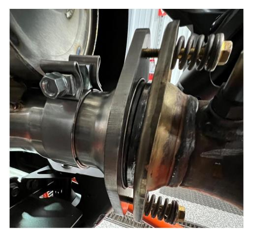
Step 10: Install the tips, leave them loose so you can move them around. Once lined up, tighten down.
