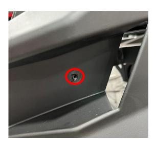
**Step 4:** Remove (2) T-50 bolts holding the rear valence on. (There are 2 metal clips above plastic)
