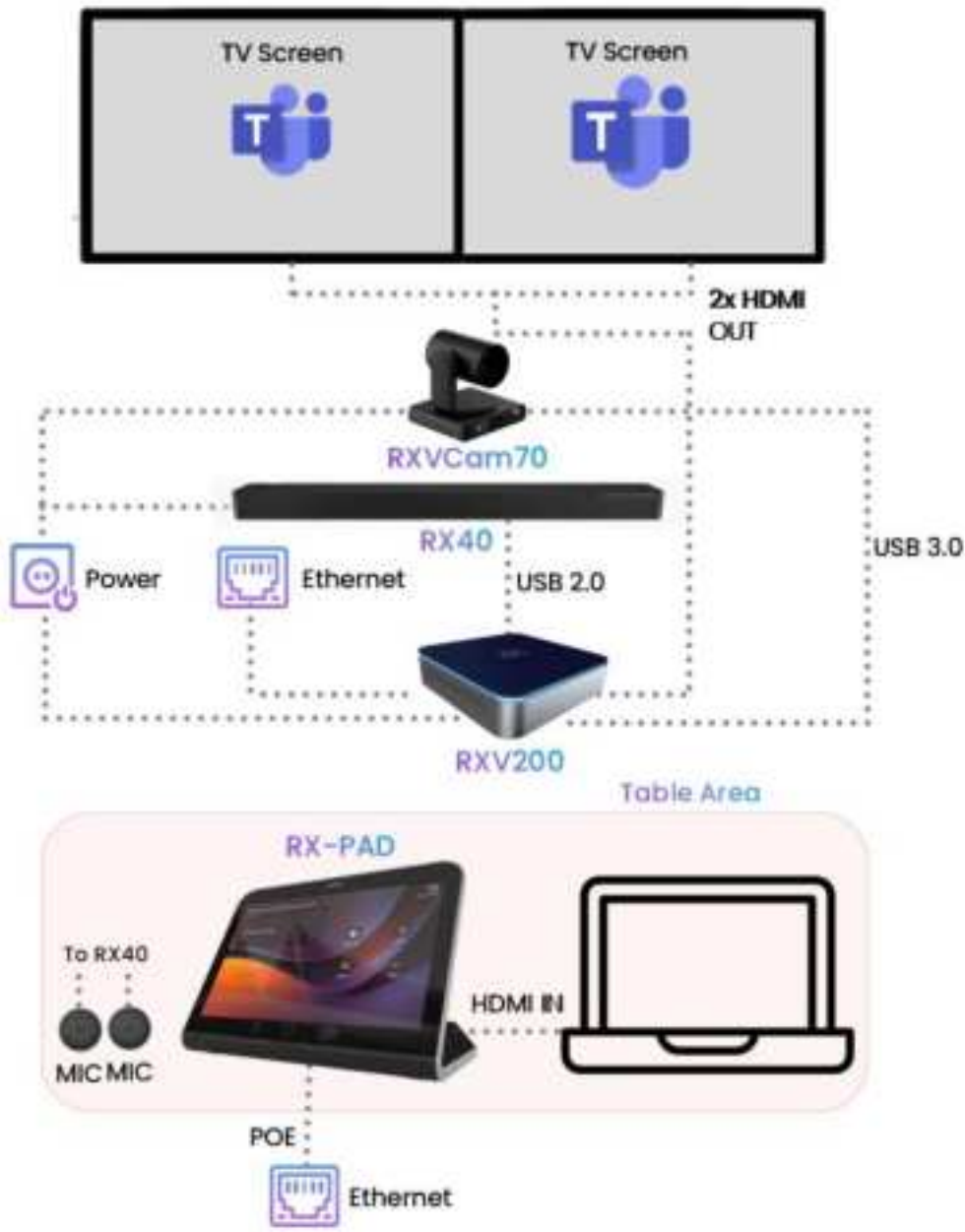
Connection Diagram for RXV200-B70
