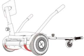
4. **WARNING:** Do not over-tighten straps when you are assembling your go-kart to your scooter. Ensure that the go-kart is secure to the scooter when attaching. Ensure the foam pads are attached to the bottom of the pedal mounts so that the go-kart does not touch the footpad sensors on the scooter. See below diagram for correct fitting.
