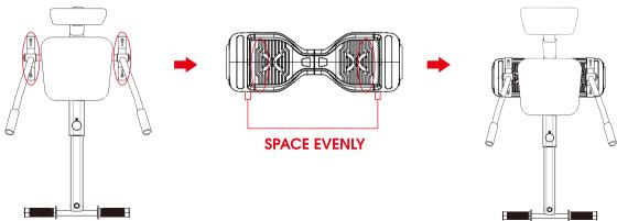
2. Secure your Hover-1 Go-Kart to your self-balancing scooter using both adjustable straps with rubber protectors. Attach one end of each strap to the holes on the front of each pedal mount as shown below.
