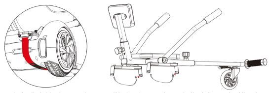
3. Wrap one set of adjustable straps under your self-balancing scooter and attach the ends of the straps on the back of each pedal mount. The rubber protectors on the straps should be centered underneath the scooter, with side B facing the ground.
