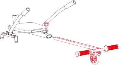
4. Insert the seat back frame into the seat frame. Adjust to preferred length. Secure the seat back frame in place using one twist knob.
