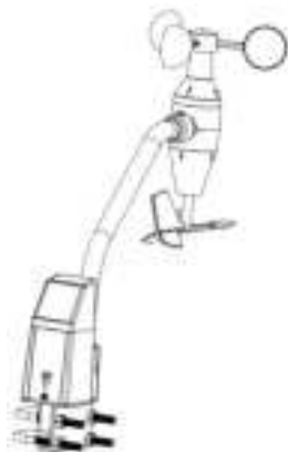
Figure 3: U-Bolts and nuts installed
