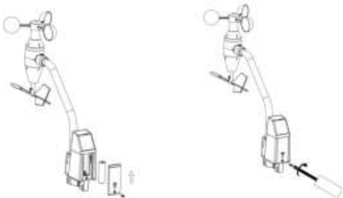
Figure 6: Battery installation diagram
