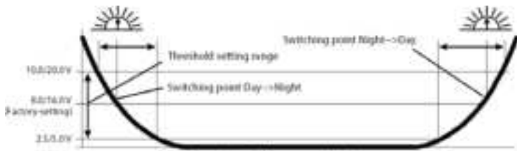
Open circuit voltage curve of solar array
