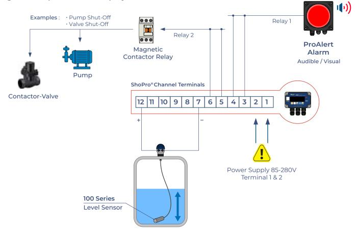
Shielded cable is recommended for control loop wiring. Use the Red wire as the (+) and the Black wire as the (-).
