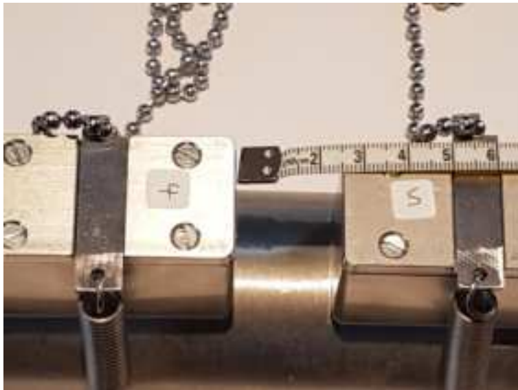
Figure(3) Flow transducer mounting, spacing is 25mm between front faces.
