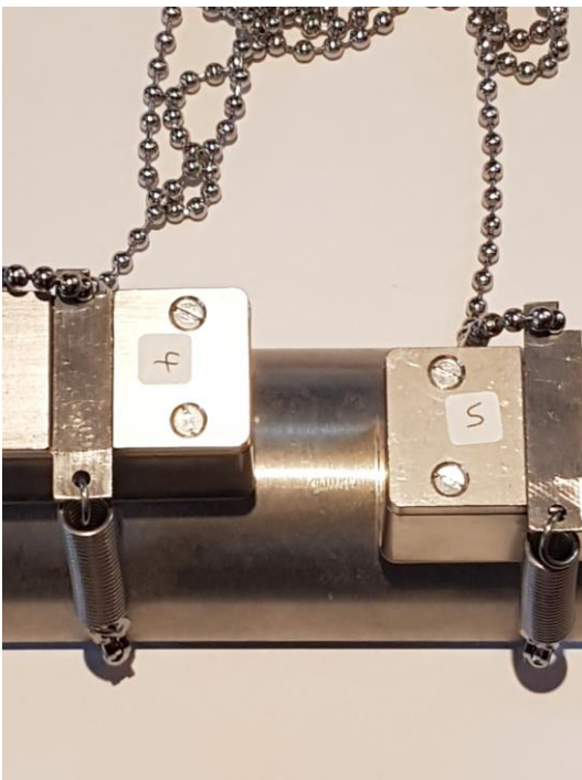
Figure(4) Misaligned transducers.
