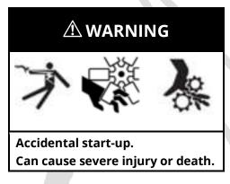
**WARNING:** Putting the generator set in AUTO mode may cause the generator set to start without warning. This can result in severe injury or death.
