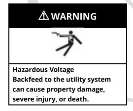
Whenever the generator set is connected as standby power, a transfer switch is required to prevent electrical backfeed into the utility electrical grid. Electrical backfeed is illegal and can result in the severe injury or death of utility company personnel working on power lines. The generator set must be installed following local, state, and National Electric Code (NEC) guidelines.
