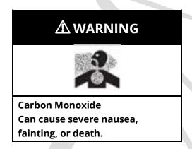
During operation, the generator set will release engine exhaust into the surrounding atmosphere. This exhaust contains carbon monoxide, an odorless, colorless, tasteless, nonirritating gas. The inhalation of carbon monoxide, even for a short period, can result in death. To reduce the risk of carbon monoxide poisoning:
