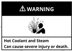
During operation, some components of the generator set can become extremely hot. These parts include, but are not limited to, the engine, exhaust manifold and piping, muffler, generator end, and voltage regulator. In addition, the engine coolant can become extremely hot and cause pressure to build up in the cooling system. Removing the pressure cap, before allowing the generator set to cool down, could cause hot coolant and/or steam to be released, resulting in severe injury or death.
