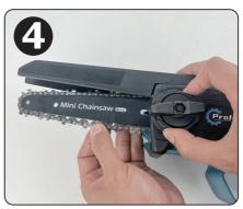
Clockwise spin the chain tension knob to adjust the tightness of the chain.
