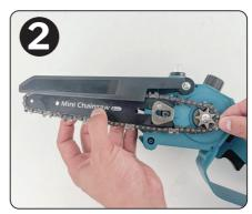
The middle guide is just clamped into the guide groove of the guide plate.
