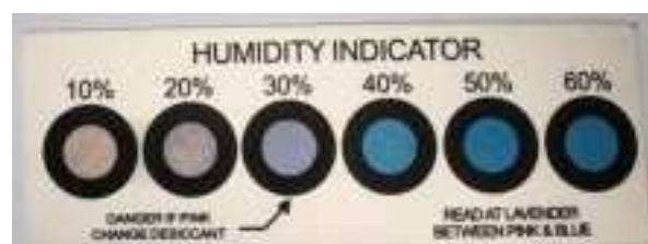
Figure 5-5 Abnormal Humidity Indication
