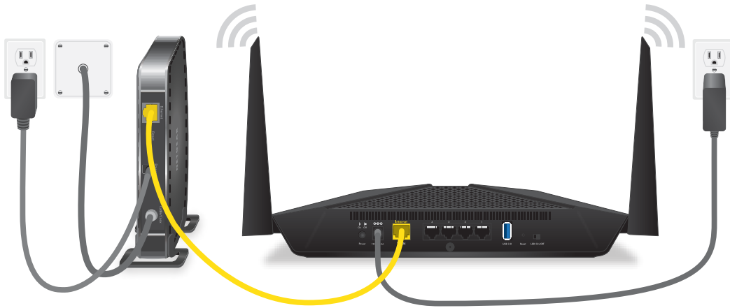
Figure 5. Cable your router
